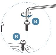
Attach mechanism (C) to the seat with  $4 \times$  screws (B), tighten with a allen key.
