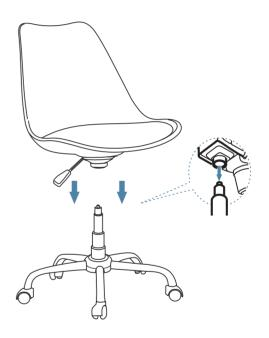
Attach the mechanism to the gas lift.
